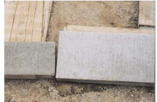
*IS blended cement (33 percent slag content) was used to produce a noticeably lighter concrete masonry unit on the right.*
