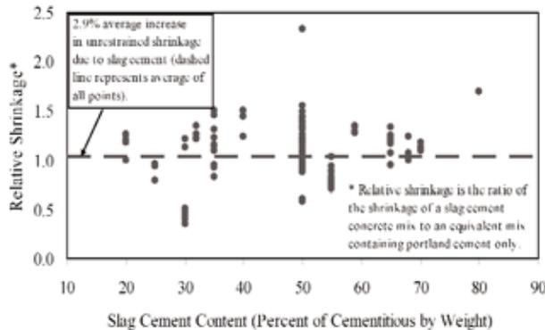
*The literature today indicates there is little increase in drying shrinkage when slag cement is used in concrete, regardless of the percentage used.*
