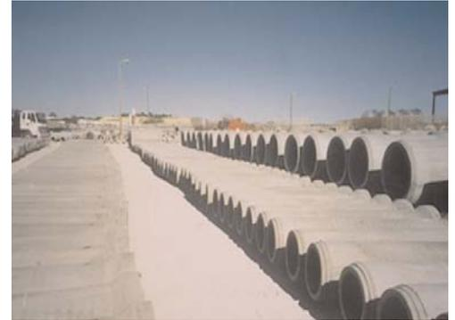
*Stockpiled concrete pipe, manufactured with slag cement.*
