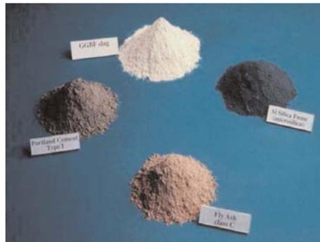
Figure 5: Comparison of various finely divided cementitious materials (Clockwise, from top: slag cement, silica fume, fly ash and portland cement).
