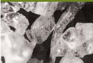
Microscopic slag cement illustrating its glassy nature
