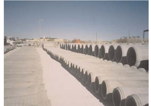
Stockpiled concrete pipe, manufactured with slag cement.
