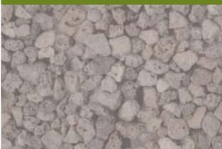
*Air-cooled slag aggregate (non-cementitious)*
