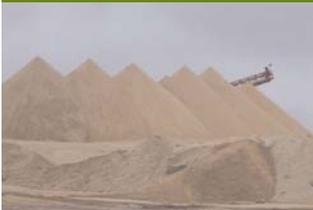
*Slag granules stockpiled and awaiting grinding.*
