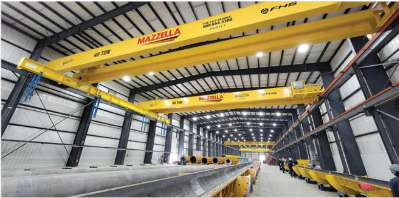
Valmont Utility worked with Germany's B+S Engineering GmbH on mold inventory and spreader bar components for the Bristol operation. Two pairs of 40-ton bridge cranes, plus a 10-ton jib crane, handle iron and fresh or hardened concrete along more than 600 feet of fully enclosed production area at the new Indiana facility. Molds travel the length through preparation, reinforcing, pour, curing chamber and stripping stations. Cured poles are staged for inspection and finishing, then transferred laterally to a rail-mounted electric cart for picking by a gantry in the sheltered, open air bay (opposite page).
