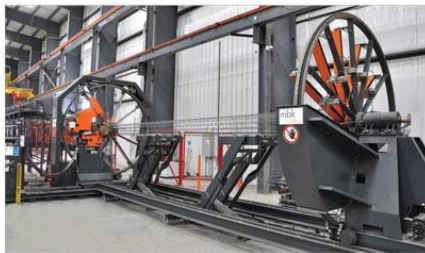
The Bristol plant is Valmont Utility's first to deploy MBK automated cage fabrication machinery. Initial performance suggests the investment is adding up to a savings of three manhours per pole versus alternative manual methods. The Indiana plant is also the producer's first to deploy a Comblift Combi-SL (Side-loader) forklift truck, whose four-way operating mode eases reinforcing bar and coil handling.
