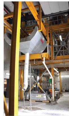
Haarup North America Inc. configured the batch plant around a Haarup 3750 counter-flow mixer. It feeds a bucket that shuttles low-slump pole mixes to a pour cart traveling the length of the molds. Haarup NA tailored the wash station shown above to turn the bucket 180° and ease cleaning of the vessel. The company also delivered fully galvanized supports and components for belt conveyors. Long-life galvanized steel is a standard for Haarup, but also a staple in products throughout Valmont Infrastructure and Agriculture segment businesses.
