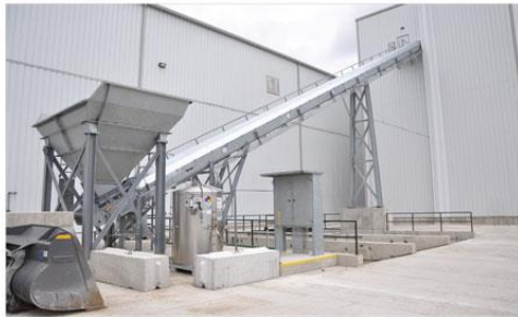
Haarup North America Inc. configured the batch plant around a Haarup 3750 counter-flow mixer. It feeds a bucket that shuttles low-slump pole mixes to a pour cart traveling the length of the molds. Haarup NA tailored the wash station shown above to turn the bucket 180° and ease cleaning of the vessel. The company also delivered fully galvanized supports and components for belt conveyors. Long-life galvanized steel is a standard for Haarup, but also a staple in products throughout Valmont Infrastructure and Agriculture segment businesses.
