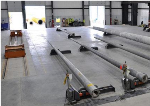
Valmont Utility worked with Germany's B+S Engineering GmbH on mold inventory and spreader bar components for the Bristol operation. Two pairs of 40-ton bridge cranes, plus a 10-ton jib crane, handle iron and fresh or hardened concrete along more than 600 feet of fully enclosed production area at the new Indiana facility. Molds travel the length through preparation, reinforcing, pour, curing chamber and stripping stations. Cured poles are staged for inspection and finishing, then transferred laterally to a rail-mounted electric cart for picking by a gantry in the sheltered, open air bay (opposite page).
